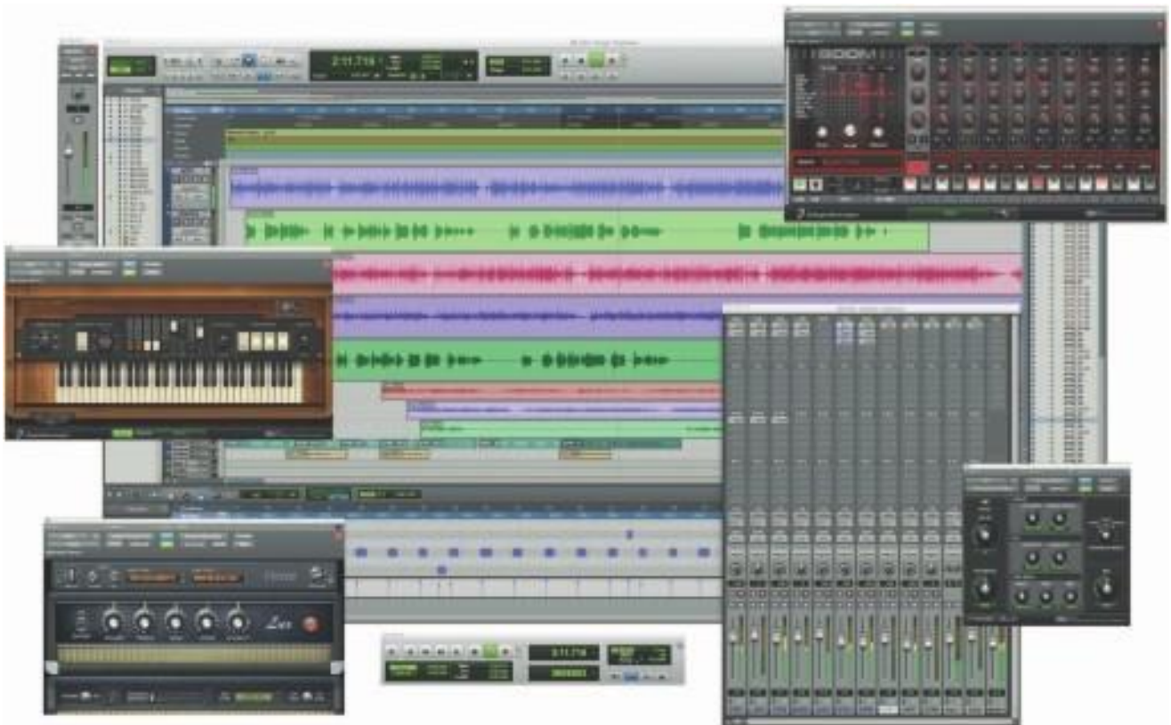
Figure 4-6 Sequencer software such as Pro Tools allows you to record, edit, and save music generated from a MIDI keyboard or instruments and blend it with digital audio.
